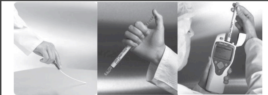
Fig. 2. Example of an ATP bioluminescence system. Note: Pictures of the 3M Clean-Trace system are used with permission from FOSS.
